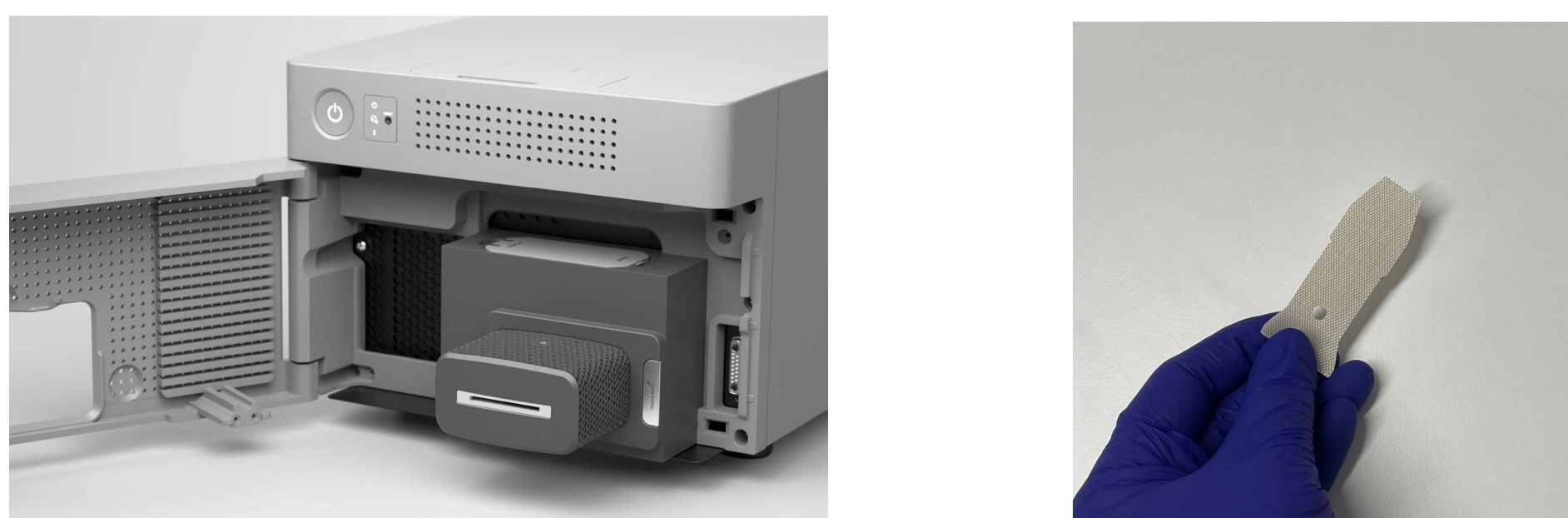
Figure 1: MSA Prototype Thermal Desorber fitted to Waters RADIANT Instrument / PTFE-coated fiberglass swabs used for sample acquisition.
