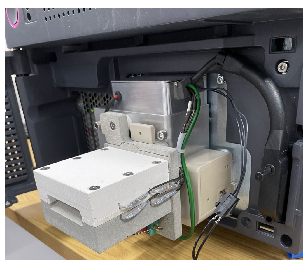
Figure 1: MSA Prototype Thermal Desorber fitted to Waters RADIANT Instrument
