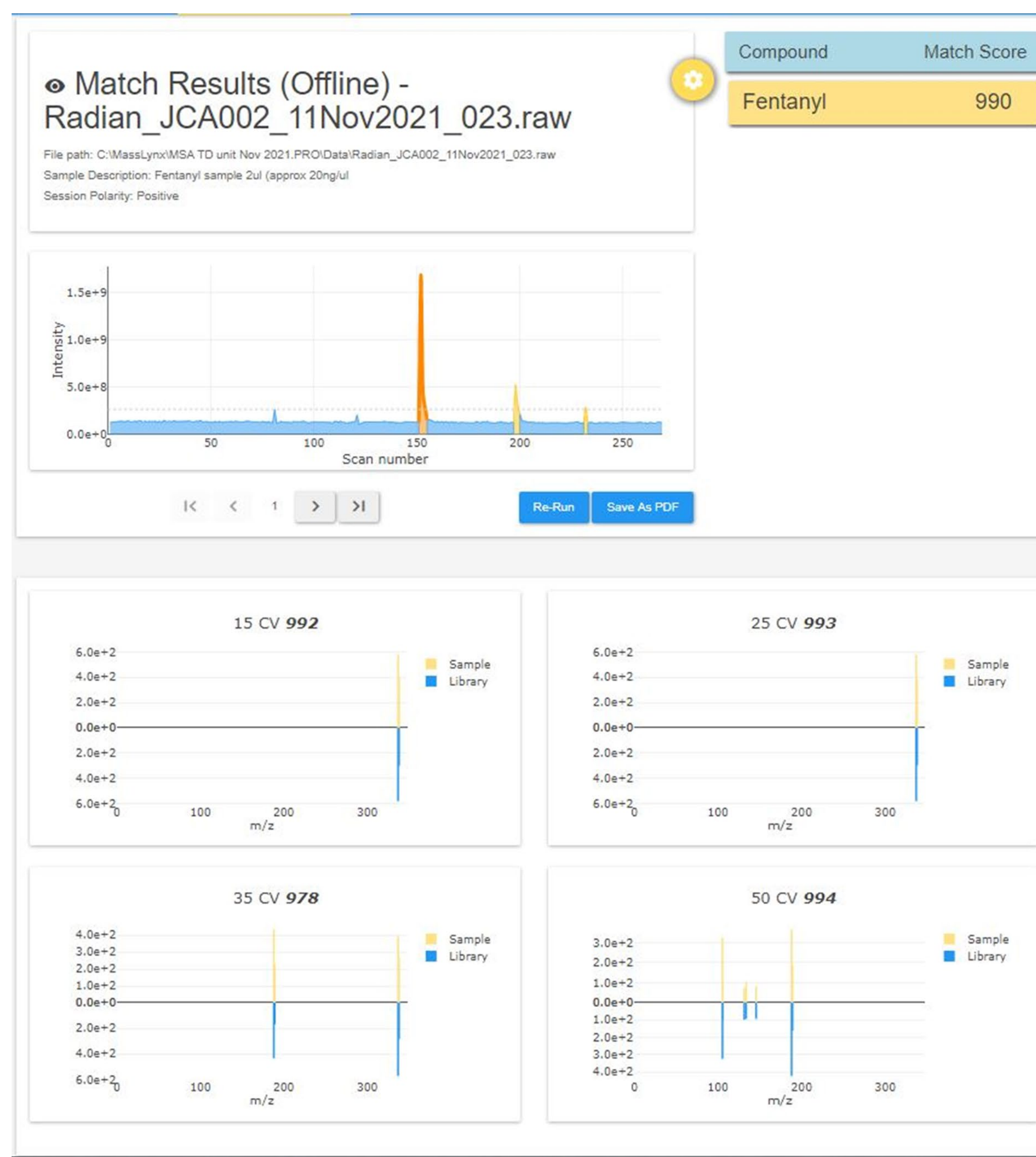
Figure 5: LiveID Sample Analysis of 2 µL Syringe Injection of 20 ng/µL Solution of Fentanyl
