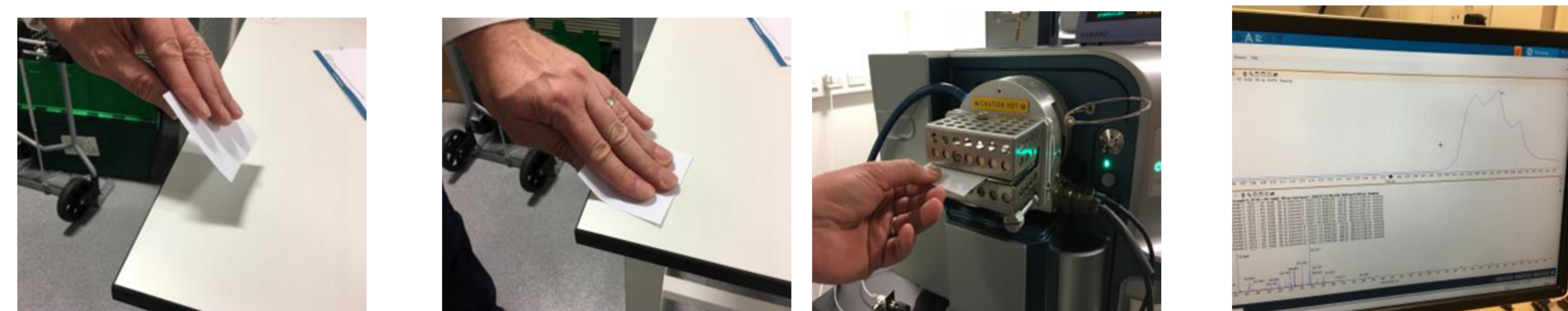
Figure 3. Images showing the deposition, evaporation, extraction and presentation of the sample to the heated blocks of the TEIS source
